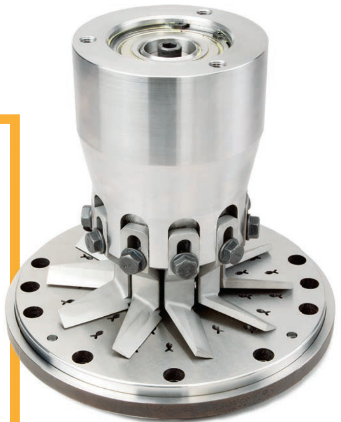
The shape and size configurations of a die plate, as well as the speed at which knives rotate around the plate, determine the size and shape of an extruded kibble or treat. Wenger
